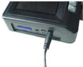
*Fig. 47 Charge main battery*
