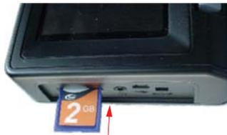
*Fig. 51 Inserting the SD memory card*
