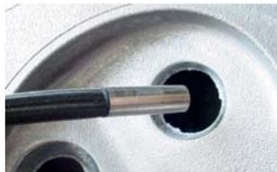
*Fig. 13 Inserting the flexible probe into the cavity*
