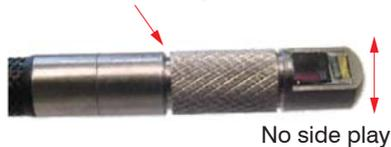
A small gap will be present when the prism tip is fully tightened in place.
