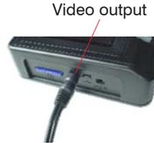
*Fig. 50 Video output on video display*
