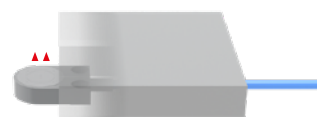
Screw mounting from below on the top side of the sensor (CSH02FL - CSH1.2FL)
