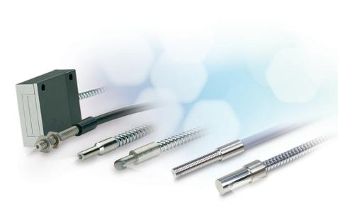
In the case of the reflex sensor, the infrared light emitted by the controller is guided to the detecting object via the sensor's fiber-optic light guides and reflected there. Both diffuse and directly reflected components are present in the back-reflected infrared light. The reflected light components of the object to be detected are received by the same sensor and transmitted back to the controller via the optical fiber for evaluation.
