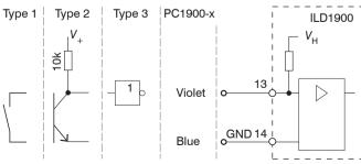
Connect the input to GND to trigger the function.
