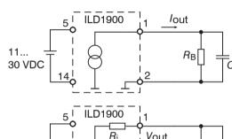
The current output may not be continuously operated in short-circuit operation without load resistor. This would lead to thermal overload and thus to the automatic overload cut-off of the output.
