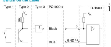
The laser remains off as long as pin 3 is not electrically connected with
