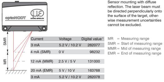
Sensor mounting with diffuse reflection. The laser beam must be directed perpendicularly onto the surface of the target, otherwise measurement uncertainties cannot be excluded.
