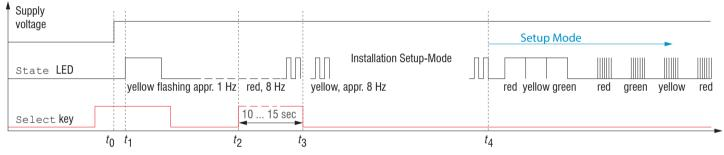
Fig. 15 Flowchart for starting a sensor in Setup-Mode
