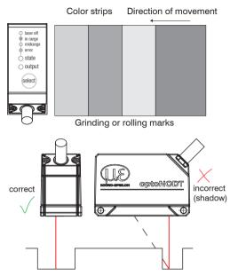
In case of rolled or polished metals that are moved past the sensor the sensor plane must be arranged in the direction of the rolling or grinding marks. The same arrangement must be used for color strips.
