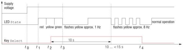
Fig. 14 Flow chart to restore factory setting
