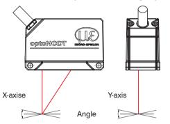
Fig. 6 Measurement errors through tilting with diffuse reflection
