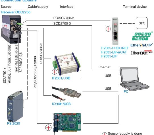
Fig. 11 Connection examples on the optoCONTROL 2700-40
