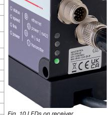
Fig. 10 LEDs on receiver
