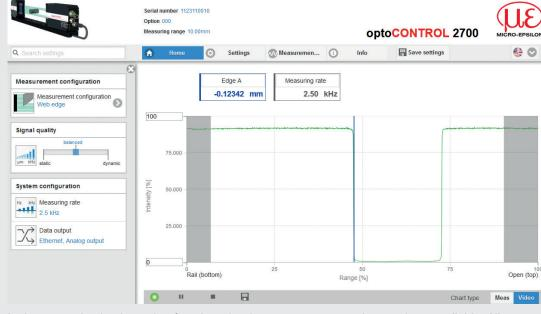
In the top navigation bar, other functions (settings, measurement chart etc.) are available. All settings on the web page are implemented in the sensor immediately after clicking the Save settings button. Parallel operation with web browser and ASCII commands is possible; the last setting
