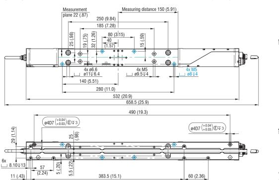
Fig. 2 Light source and receiver ODC2700-10, ODC2700-40 with mounting rail, dimensions in mm (inches)
