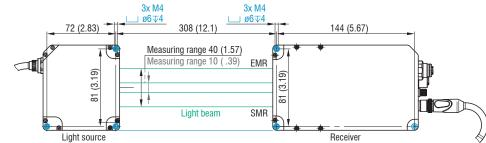
Fig. 5 Mounting thread for direct fastening ODC2700-10, ODC2700-40, dimensions in mm (inches)
