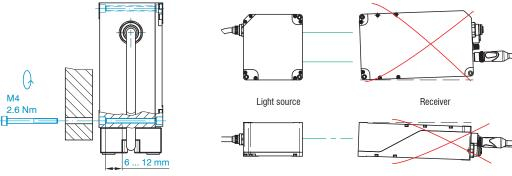
Fig. 6 Direct fastening of sensor
