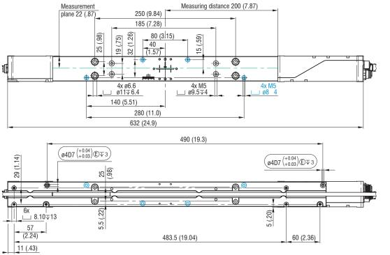
Fig. 4 Light source and receiver ODC2700-40(002) with mounting rail, dimensions in mm (inches)
