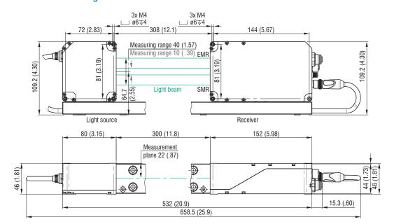
Fig. 1 Light source and receiver ODC2700-10, ODC2700-40, dimensions in mm (inches)
