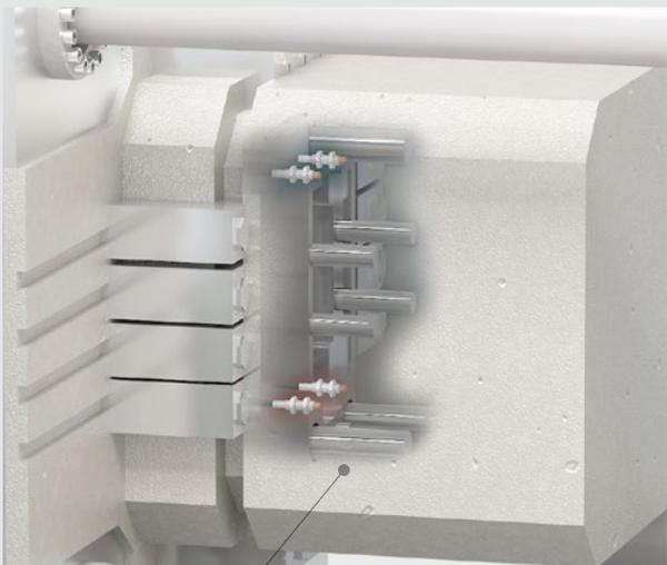
Gap measurement in aluminum die-casting molds
