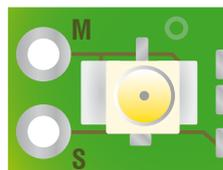
S = signal = inner conductor
