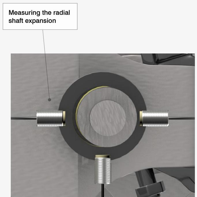
Environmental influences such as oil, temperature, pressure and moisture are largely compensated for and have a minimal effect on the signal. For this reason, the sensors are ideal in demanding application areas, such as industrial mechanical engineering and test bench construction.
