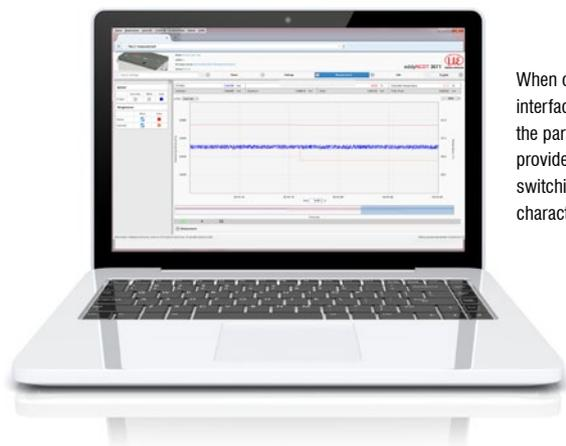
When connecting a PC via the Ethernet interface, a modern web interface can be accessed without any further installation and enables the parameterization of sensor and controller. The DT3071 controller provides enhanced features such as 5-point calibration, setting of switching and temperature outputs, as well as storage of multiple characteristic curves.
