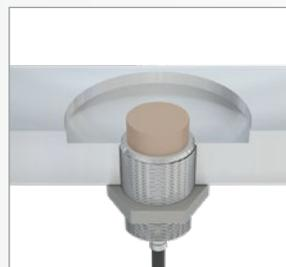
**F Installation of unshielded sensors with a recess**
