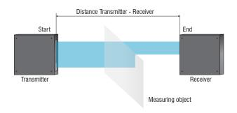
Transmission sensor with transmitter and receiver
