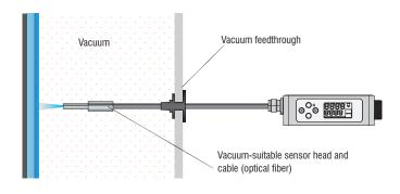
The fiber optic sensors and fiber optic cables are built with passive components and do not emit heat to the environment. In vacuum, sensors (temperature bonding T250), optical fibers (stainless steel sheath), and the vacuum feed-through up to 10<sup>-5</sup> mbar can be used.
