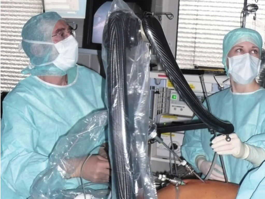
With the non-leading hand, the surgeon controls the movements of the system with the wireSENSOR units, accurate to a few millimetre
